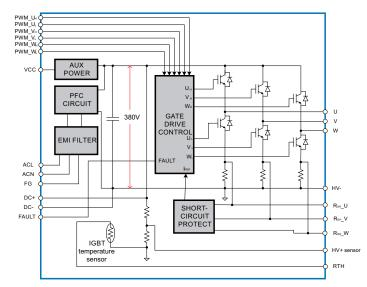
DC input type : VFD-150P-48/ VFD-250P-48/ VFD-350P-48
