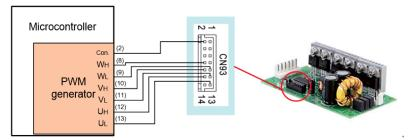
Note that simultaneous activation on the high-side (H) and the lowside (L) switches on the same phase is prohibited. A switching control signals dead-time ( $t_{dead}$ (Min.)) of 300ns or above is required.
